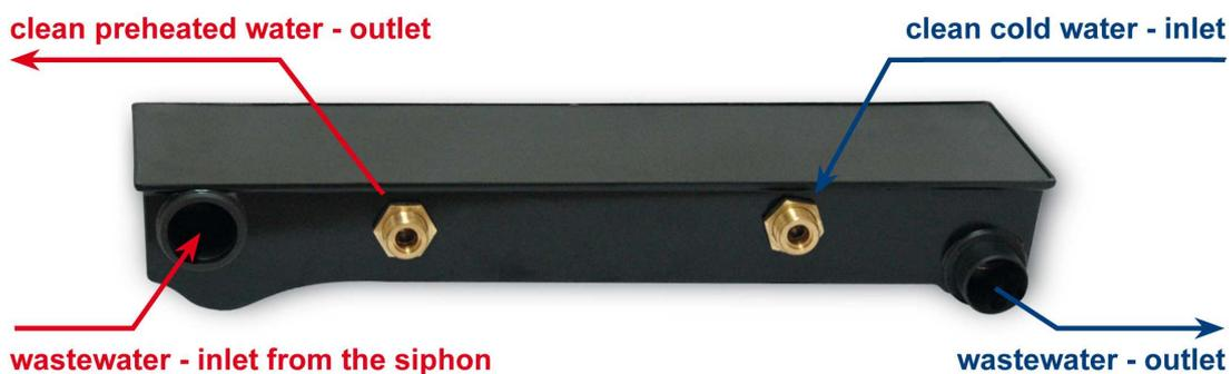
The heat exchanger is designed for wastewater heat recovery in bathrooms up to the water maximum pressure of 16 bar and temperature up to 90°C. It is not appropriate to tread on the exchanger.
