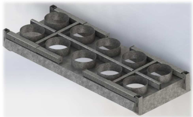
Filling bench dismantled for its transport
